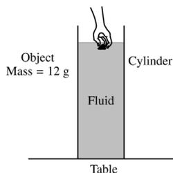
In an experiment, students used video analysis to track the motion of an object falling vertically through a fluid in a glass cylinder. The object of  $m = 12\text{ g}$  is released from rest at the top of the column of fluid, as shown above. The data for the speed  $v$  of the falling object as a function of time  $t$  are graphed on the grid below. The dashed curve represents the best fit chosen by the students for these data.
